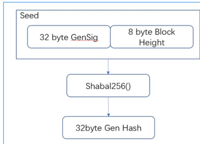
Now, the miner will do a small mathematical operation on this hash to find out which scoop number to use when processing the plot files. This is done by taking the generation hash modulo 4096, as there are only that many scoops.
