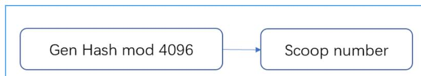
Next step for the miner is to read all the 64-byte long scoops from all nonces in all plot files. It will process them individually through shabal256 together with the new generation signature to get a new hash called target. This target is now divided with base target and the first 8bytes of the result is the value deadline.
